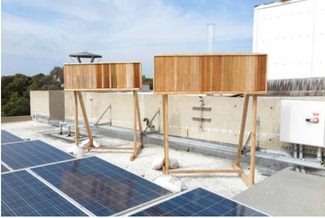
During the project mock-up phase, different finishes were trialed on sample panels of existing weathered (left) and new (right) teak Photo: J. Paul Getty Trust
