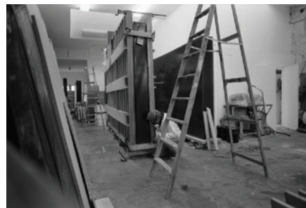
10. The wider end of the mold in which the resin has been cured has been removed and De Wain Valentine is inspecting the base of one of the polyester slabs. Photo: Courtesy of De Wain Valentine Artwork: © De Wain Valentine
